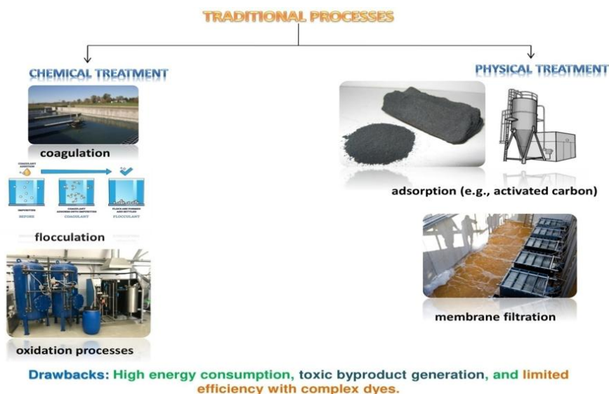
Figure 1. Framework of Traditional Dye Remediation Processes. The chemical treatment process is depicting coagulation, flocculation, and oxidation processes and physical treatment process showing adsorption and membrane filtration.
